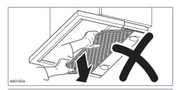
When removing the grease filter do not tilt it downwards at an angle.
